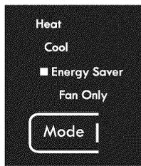
You will save energy usage in this mode. The compressor and motor will turn off once the room is at the desired temperature. The air will be sampled for 20 seconds every 10 minutes until the room is above the set temperature, at which point the compressor turns back on and the fan runs. The entire process is now repeated.
